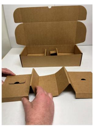
With the recycled (less smooth) side upwards, fold in the side flaps
